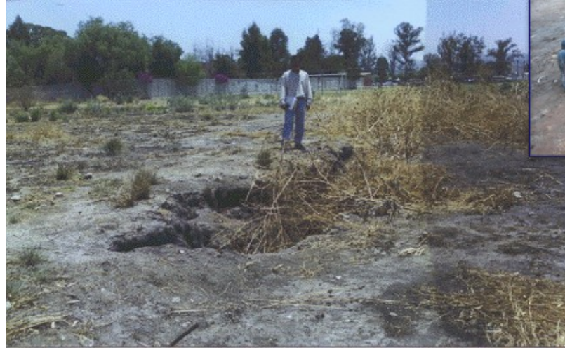
Tensional open fracture without significant vertical displacement
