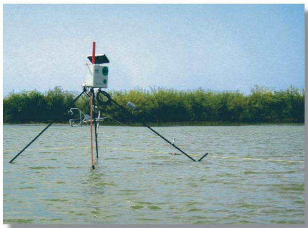
DEVICE FOR THE MEASUREMENT OF EVAPORATION THROUGH TURBULENT CORRELATION
